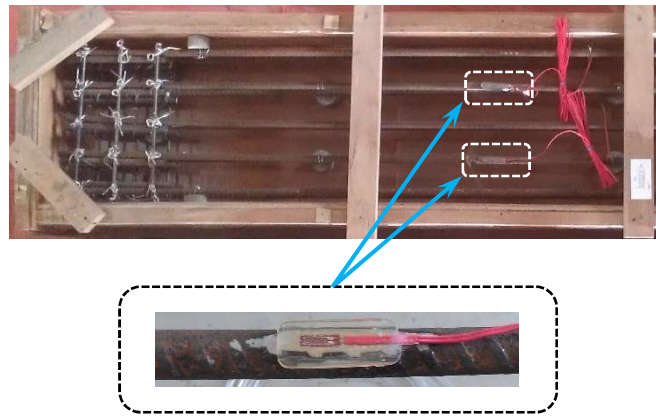
Figure 5: Strain gauges on longitudinal steel.
