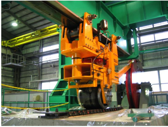
(a) Experimental set-up for cyclic moving wheel loads
