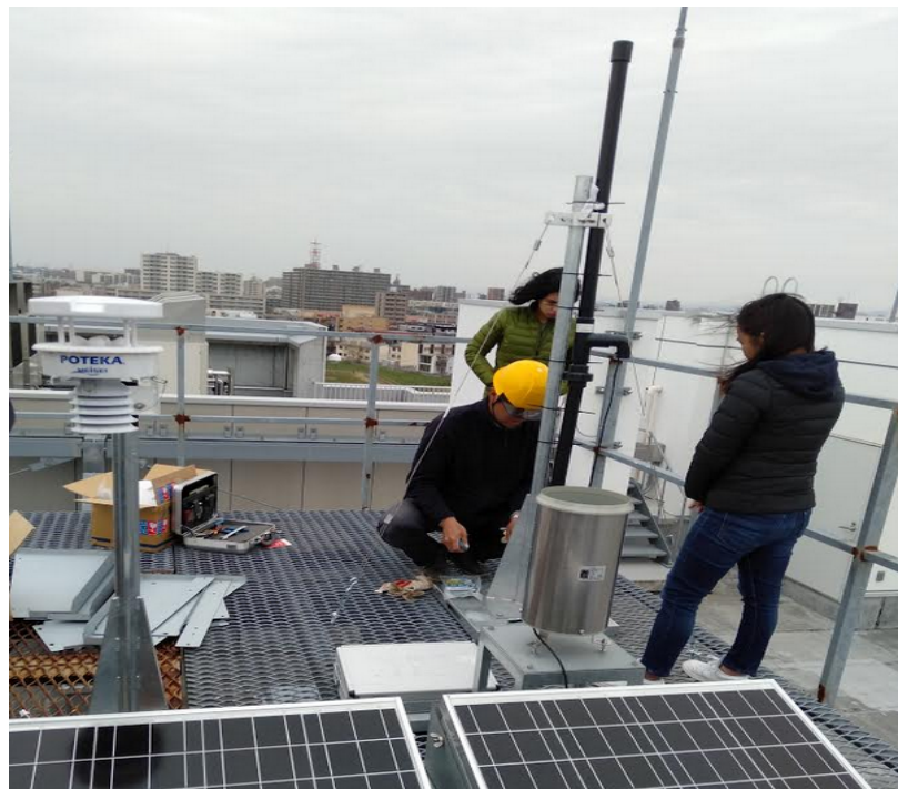
Figure 2.3. Example of V-POTEKA installed on roof top building of Hokkaido University. This kind of V-POTEKA is distributed to Philippines as Philippines Nation-wide Network
