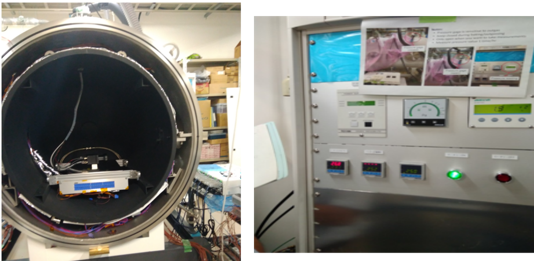
Figure. 3.6. TIS camera is tested in vacuum chamber
