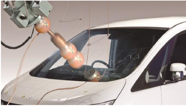
Figure 9. Impact test for assumption of pedestrian head, [14]
