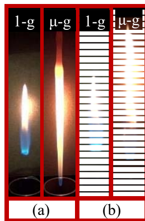
Figure 4. Flames images in normal- and micro-gravities for (a) ( U_F [m/s], U_A [m/s]) = (6.37, 0.5) and (b) (10.6, 0.5).
