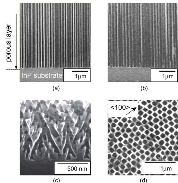
**Fig. 4** SEM images of  $\langle 001 \rangle$ -oriented straight nanopore arrays: (a) the cross-section of straight nanopores obtained in Electrolyte B, (b) the cross-section of straight nanopores obtained in Electrolyte C, (c) nanopores with  $\langle 113 \rangle$ -oriented branches obtained in Electrolyte A at  $V_s = 2V$  and (d) plan view of InP nanopores formed in Electrolyte B.
