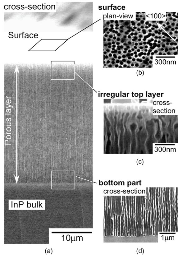
**Fig. 3** SEM images of wavy porous structures formed in Electrolyte A under  $V_s = 5V$  and  $t_a = 1min$  with light illumination. (a) Overall structure, (b) surface, (c) irregular top layer and (d) bottom part.
