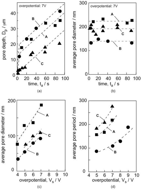
**Fig. 5** The measured data of (a) pore depth vs. time, (b) average pore diameter vs. time, (c) average pore diameter vs.  $V_s$  and (d) average pore period vs.  $V_s$  obtained by cross-sectional SEM observation.
