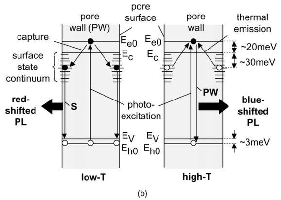
**Fig. 6** (a) PL spectra taken from nanopores formed in Electrolyte C at various measurement temperatures, showing presence of pore wall (PW) and surface state (S) components, and (b) a model for energy levels and radiative transition processes for PW and S emissions. The dashed curve in (a) shows PL peak positions of InP band edge emission.
