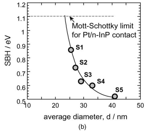
**Fig. 9** SBH values of various InP Schottky contacts; (a) metal work function dependence of SBH and (b) SBH values plotted vs. average particle diameter,  $d$ . S1 - S5 correspond to those in Fig. 15.
