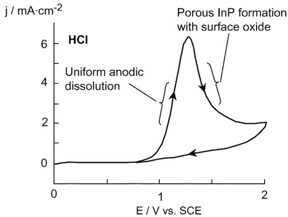
**Fig. 1** Cyclic voltammogram of n-InP in a dilute HCl solution with pH of a 1.0 in the dark.
