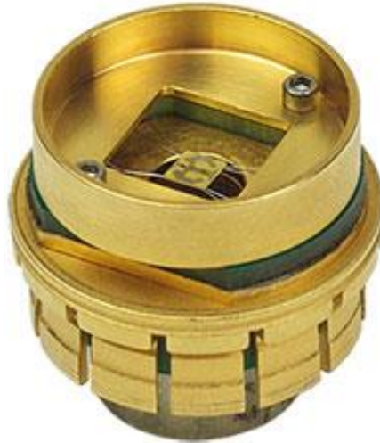
Figure 2.7. Calorimeter puck for heat capacity measurement.
