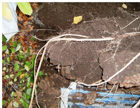
Figure 3. The bent tip of horizontal root with the 30-cm treatment. The arrow indicates where the root-barrier panel was set.
