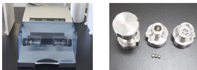
Supplementary Figure 1. Retsch MM400 mill (left) and ball milling vessels (right).
