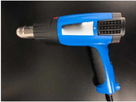
Supplementary Figure 3. Temperature-controllable heat gun used in this study.
