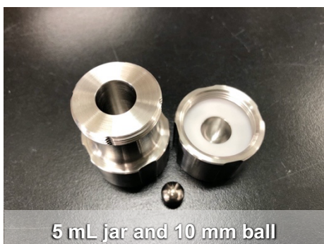
Supplementary Figure 2. Stainless jars and balls used in this study.
