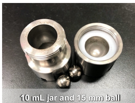
Supplementary Figure 2. Stainless jars and balls used in this study.
