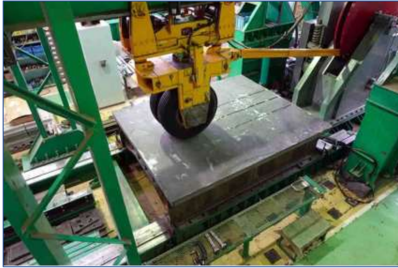
Figure 1.1 Fatigue test of full-scale OSD reinforced with UHPFRC overlay [9]
