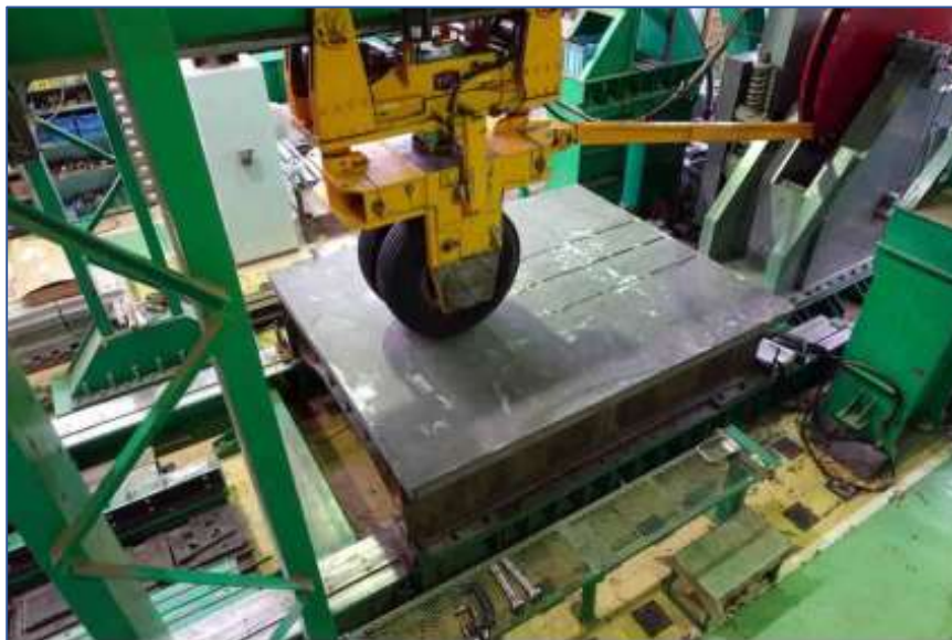
Figure 4.1 Fatigue test of full-scale UHPFRC-steel composite bridge deck in stage 1 subjected to a moving wheel loading with rubber tire under dry condition. [9]
