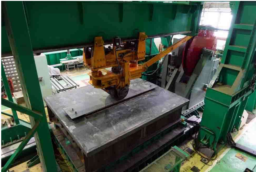
Figure 6.1 Fatigue test of UHPFRC-steel composite bridge deck in stage 3 subjected to a moving loading with steel wheel under dry condition. [9]
