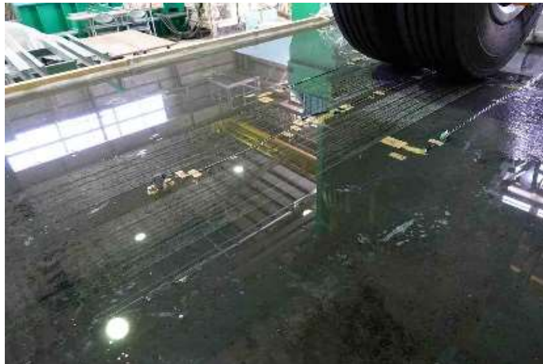
Figure 5.1 Fatigue test of UHPFRC-steel composite bridge deck in stage 2 subjected to a moving wheel loading with rubber tire under surface water condition [9]
