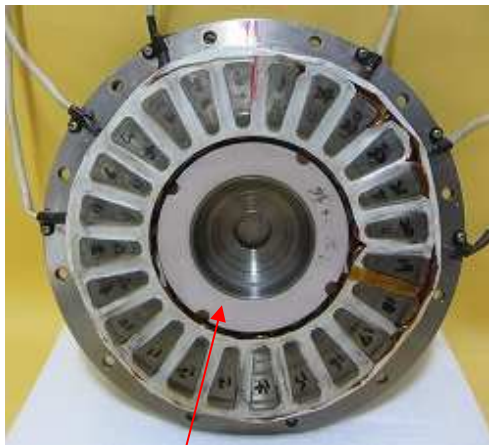
Field winding terminal
