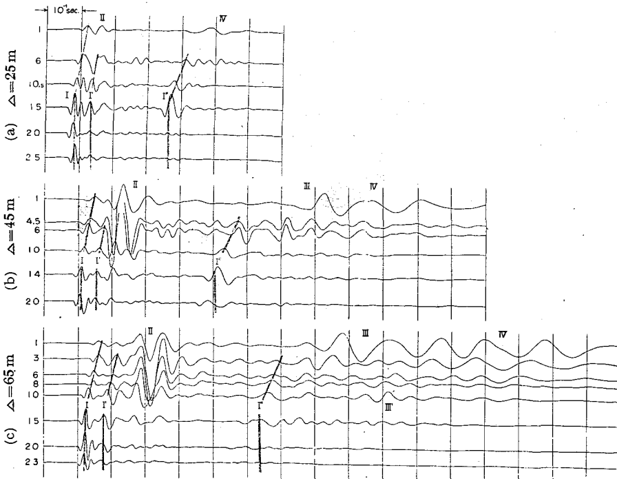
Fig. 9. (a) Seismic records at 25 m distance from shot hole. (b) Seismic records at 45 m distance from shot hole. (c) Seismic records at 65 m distance from shot hole.
