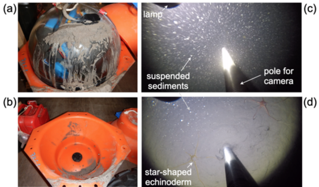
Figure 10: (a, b) Photographs of the OBS after retrieval and removal of the upper protective shell (credit: N. Kanna; August 2019). (c, d) Underwater photographs taken \sim 0.5 km from the OBS drop point and a few meters above and at the bottom of the fjord (200 m depth) during sediment coring of BF9 (diameter of the camera pole is 2.5 cm; credit: T. Ando; July 2018).
