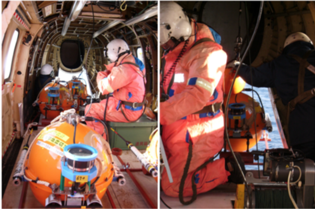
Fig. B 1: A potentially useful methodology at the calving fronts: OBS deployment from a helicopter (offshore Hokkaido, Japan; credit: Y. Murai, February, 10, 2006). The shown OBS model is larger and slightly different in design from the one used in this study.
