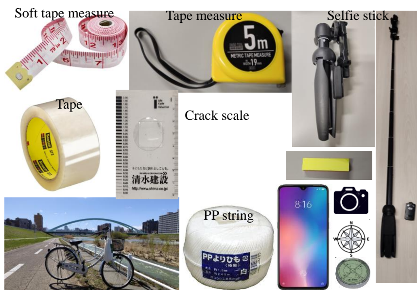
Figure 5.3 Tools used to collect onsite information for the targeted bridges
