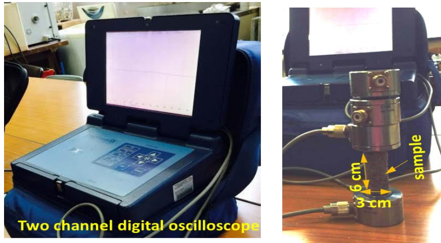
Figure 5. 7: Ultrasonic measurement of fiber treated MICP specimen.
