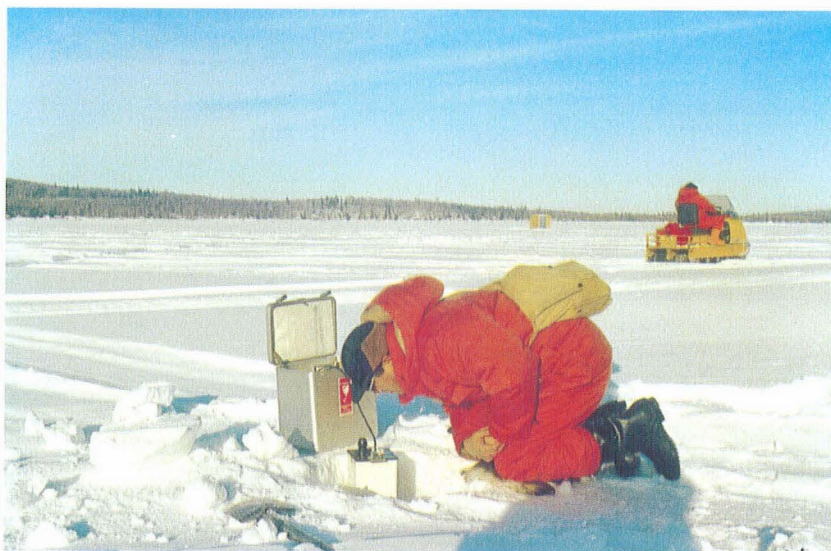
Photo. 2 Graviometric surveying by a gravimeter of LaCoste and Romberg on the covered ice of Harding Lake.
