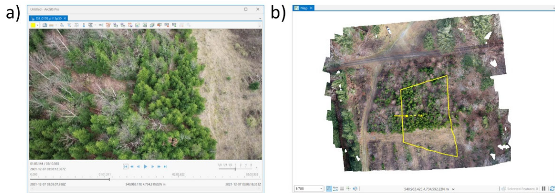
Figure 26. a) The video where I identified the fallen and snapped tree, b) GIS with the orthomosaic and the video footprint (in yellow).
