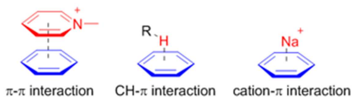
Figure 1-1. Examples of \pi - \pi , CH- \pi and \pi -cation interaction. Copy right from Wikimedia.
