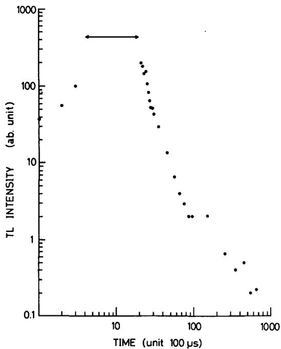
Fig. 2. Variation of TL intensity as a function of time. Data are out-of-scale during the time interval indicated by a horizontal arrow.
