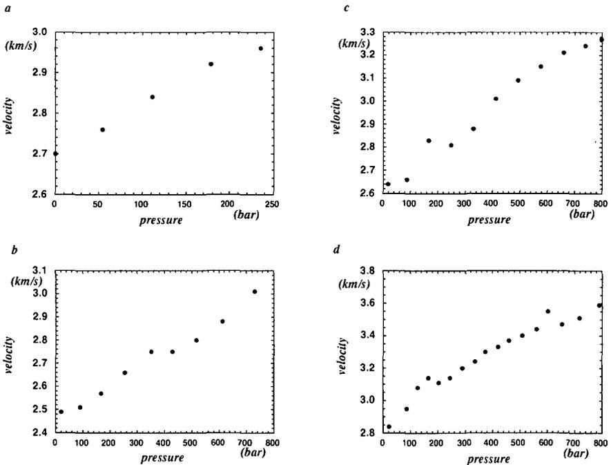
Fig. 3. The velocity variations as a function of the uniaxial stress.
