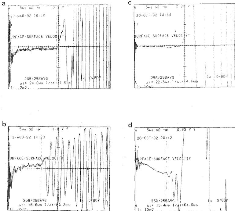
Fig. 2. The example of observed signals obtained through four devices. The stress applied is 50 to 100 bar. A broken line indicates the arrival of the first phase.
