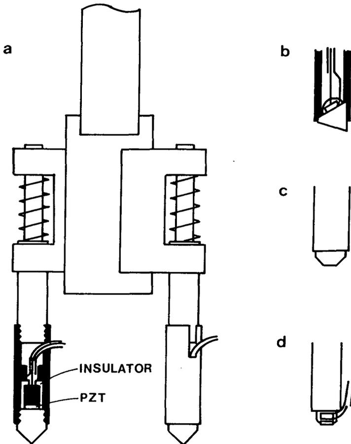
Fig. 1. The whole structure of the device *a*. The transducer rod of the devices *b*, *c* and *d*.
