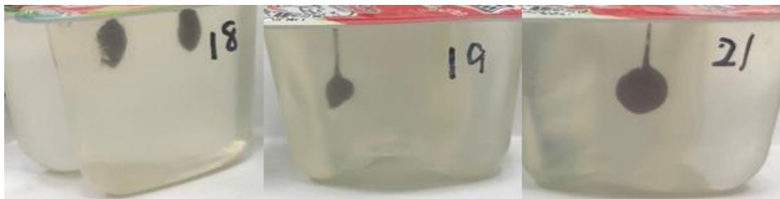
Figure S6. Biopex-Au NPs injected through 18G, 19G, and 21G needles.
