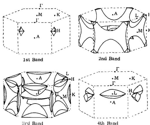
Fig. 8 The one OPW Fermi surface in the reduced zone scheme (after Harrison 1966).
