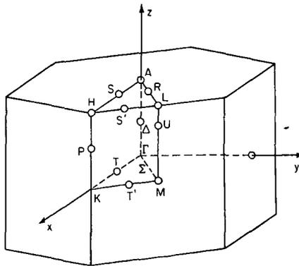
Fig. 7 The first Brillouin zone of the hexagonal closed pack structure. The names of the symmetry points are followed by Koster (1957).
