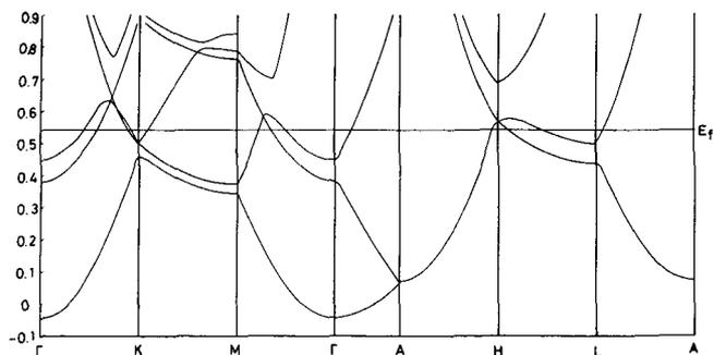
Fig. 4 The band structure corresponding to  $V/V_0=0.8$ .
