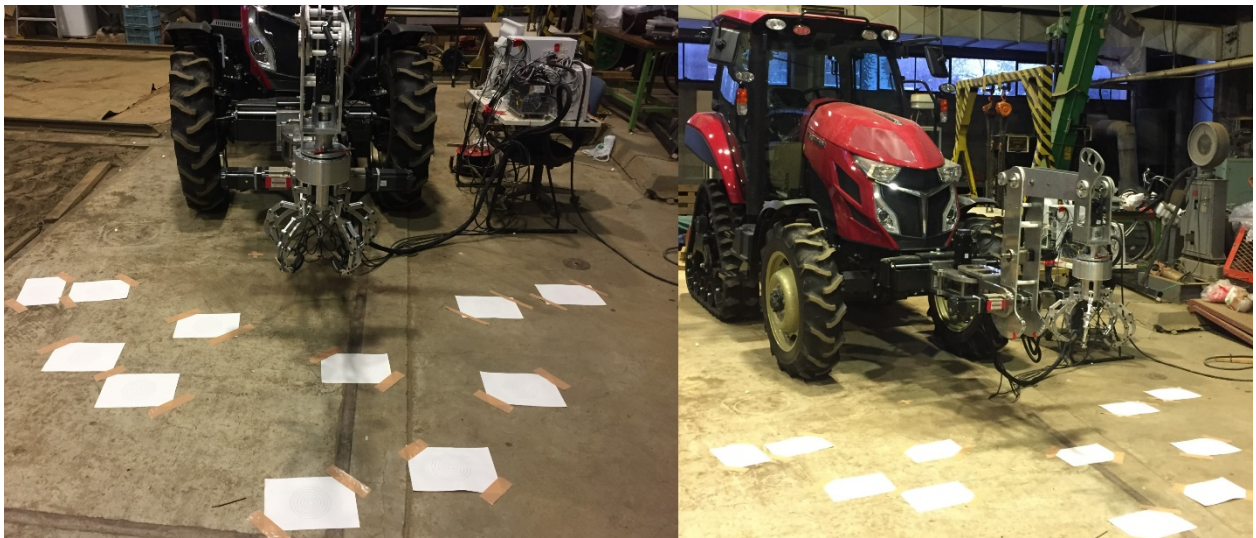
Figure 111. Accuracy and repeatability experimentation illustration, installed on robot tractor.
