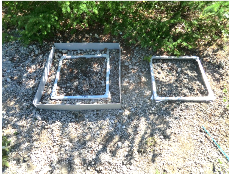
Photo 2.8 Collars were set as control (CC) (right) and trench (TC) (left) as a pair.
