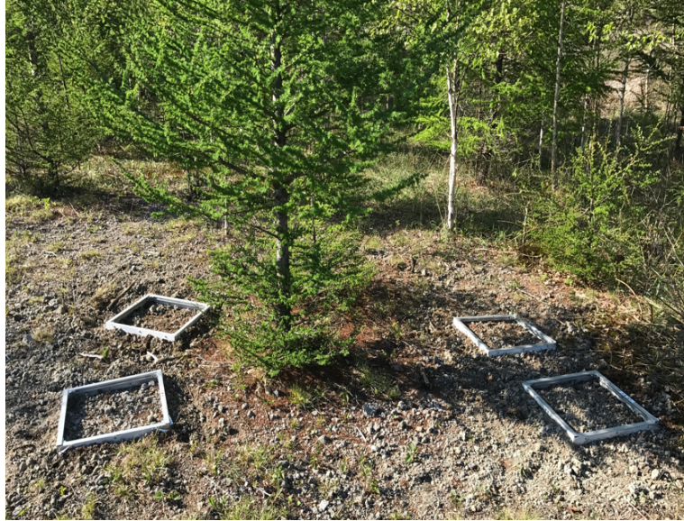
Photo 2.7 Collars were set at 0.5 m (Near), and the others were set at 1.0 m (Far) from the target larch stems.
