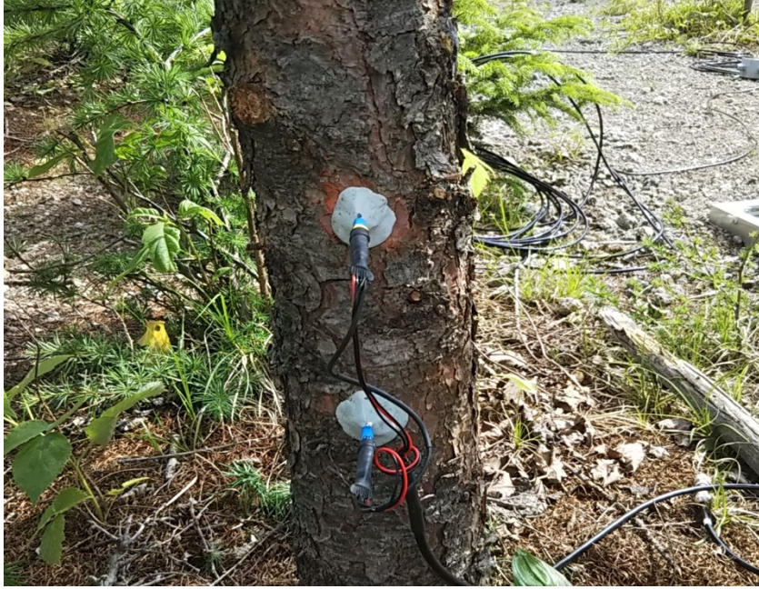
Photo 2.12 Sap flow sensor installation
