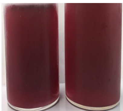
Fig. 3-3. Photograph of Au NPs' colloidal solution with average particle diameter of 30 nm (left) and 44 nm (right).
