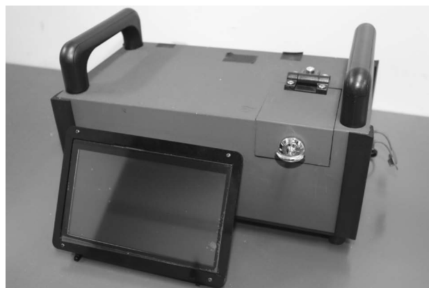
Fig. 2 Photograph of fluorescence polarization measurement apparatus
