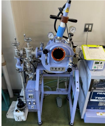
Figure 2.1 Arc melting furnace with an enclosed crucible
