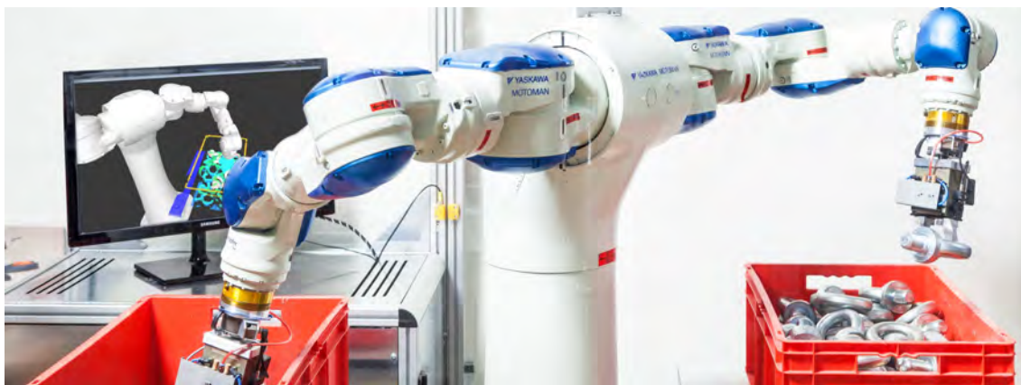
Figure 1.3: An experimental real-world robot cell from Fraunhofer IPA [13]. A dual-arm robot is taking parts out of a bin and dropping them into another.
