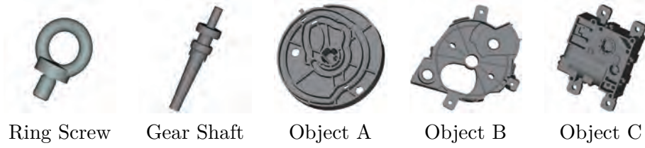
Figure 2.6: Models of objects used in the experiment. The gear shaft and ring screw are from the Fraunhofer IPA Bin-Picking dataset [13], and Object A, B, C are from XA Bin-Picking dataset [16].
