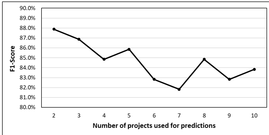
Figure 4.5: Results evaluating the relevance of the top-3 predicted and recommended mining methods using the F1-score
