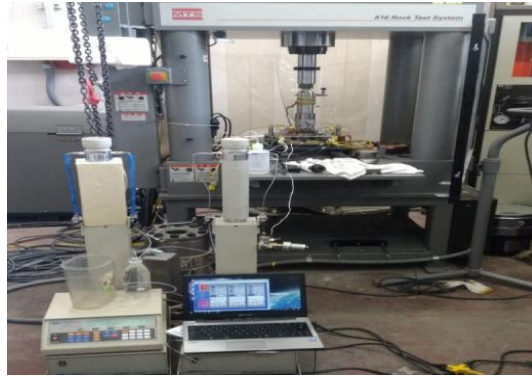
Fig 3.9 Experiment set up for triaxial test, (showing the MTS loading frame, Hokkaido University).
