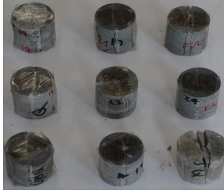
Fig 3.3 Fractured specimens after Brazilian test.
