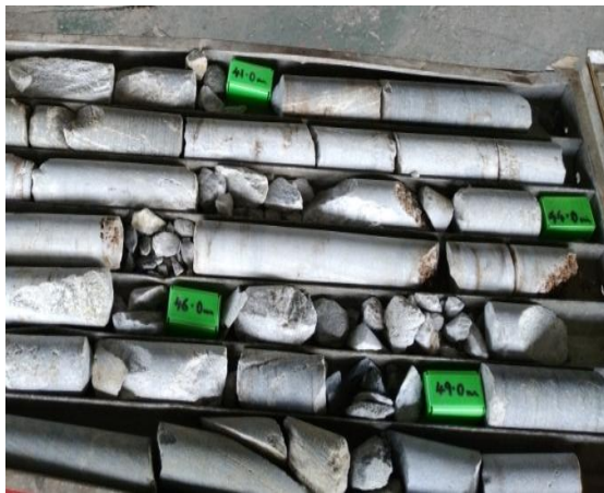
(a) Tray of drilled core from 1423 meter level.
