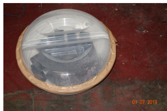
(c) Sealed container with 100% humidity.
