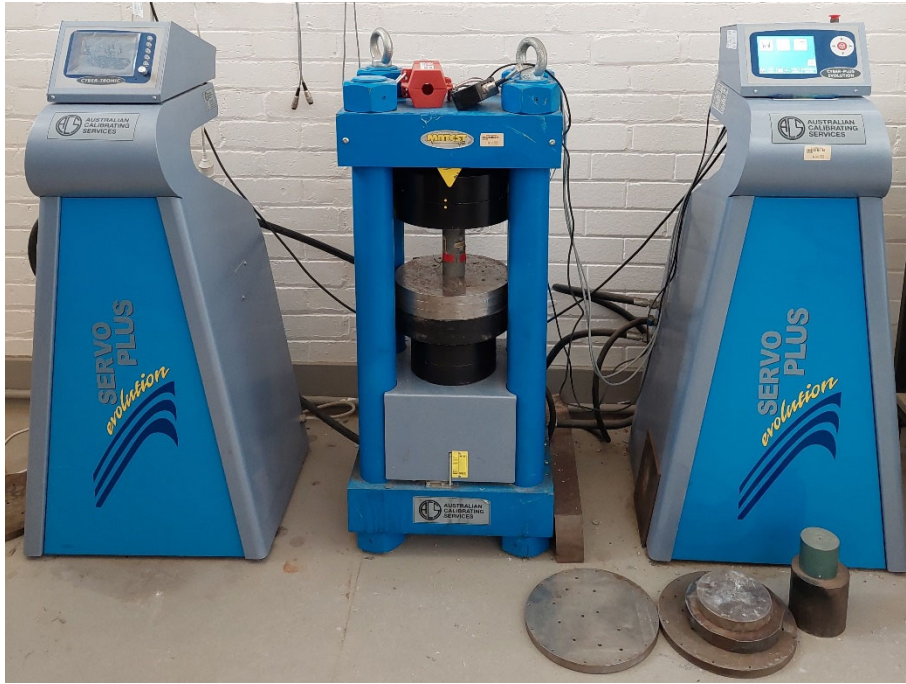
Fig. 3. Servo-controlled high stability compression testing apparatus for the UCS and BTS tests
