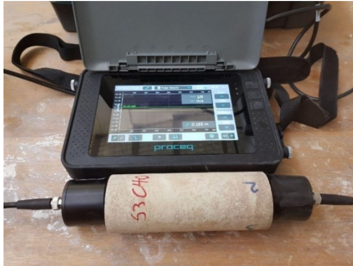
846 Fig. 1. Pundit PL-200 equipment for measuring P-wave velocities of the cylindrical rock specimens
