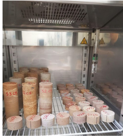
i) Climatic controlled cabinet together with a assembly of tested samples
