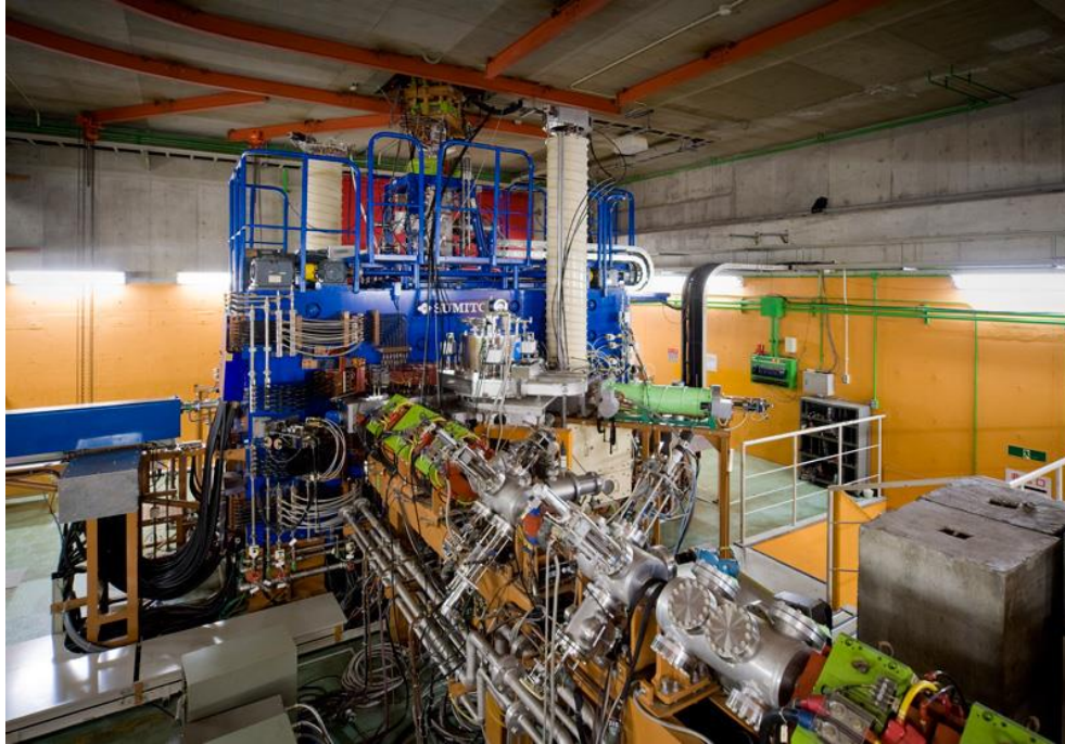
Fig. 2.1. RIKEN Azimuthally Varying Field (AVF) Ring Cyclotron
