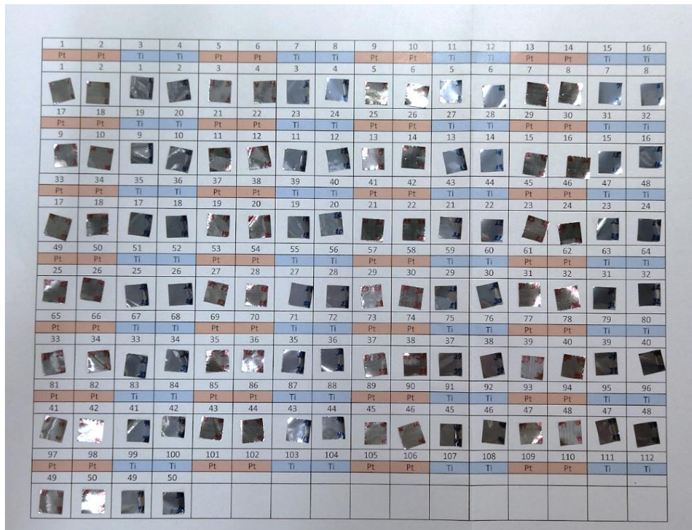
Fig. 4.1. The target configuration ( ^{nat}\text{Pt} and ^{nat}\text{Ti} foils)
