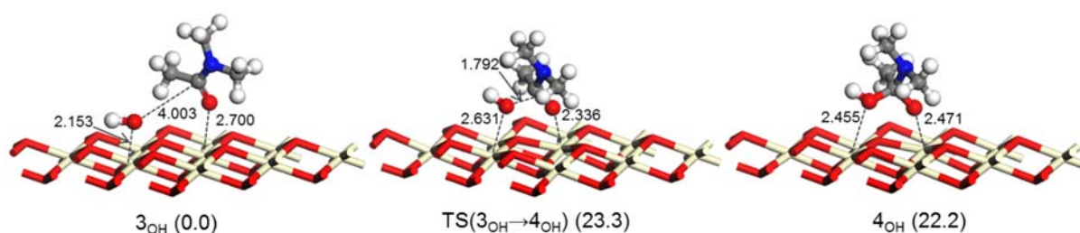
Figure 10. Optimized structures and relative energies for the nucleophilic attack of the OH group to the carbonyl carbon atom of N,N -dimethylacetamide on the CeO 2 surface. Only important part is displayed for clarity. Units in Å and kcal/mol. Color code: beige: Ce; red: O; grey: C; blue: N; white; H.
