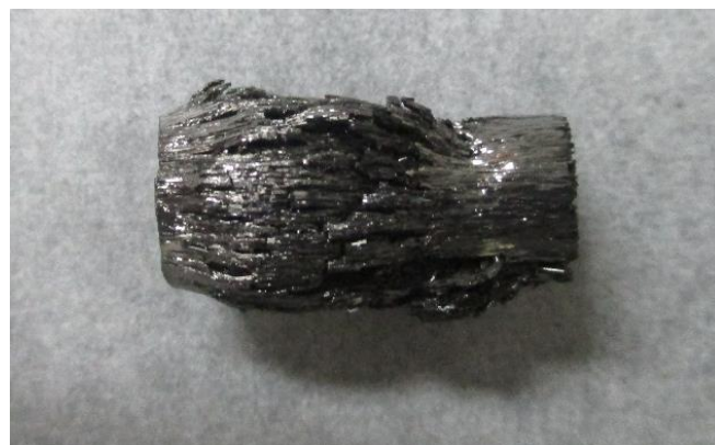
Fig. 4.5 Visual appearance of a FCGM with an expected void fraction \varepsilon_v of 0.69. Severe cracks due to fiber overload can be clearly seen
