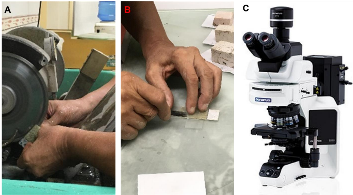
Figure 18. Thin Section Analysis. A. Cutting samples into coral blocks. B. Preparing thin sections from coral blocks. C. Petrographic analysis of corals using polarizing microscope
