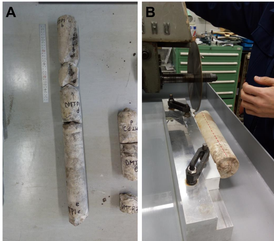
Figure 21. Cutting of coral samples using lapidary rock saw with diamond-tipped blade
