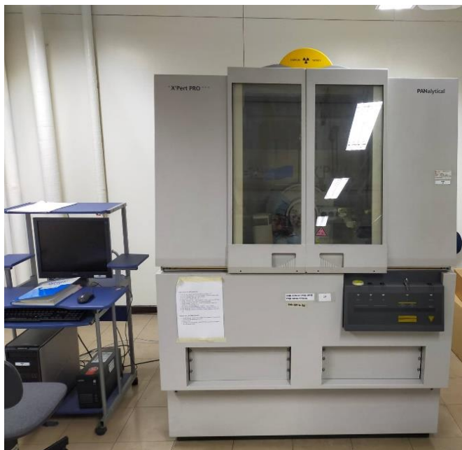
Figure 19. X-ray diffraction (XRD) Analysis. Pulverized coral samples were analyzed in X'Pert PRO PANalytical XRD.
