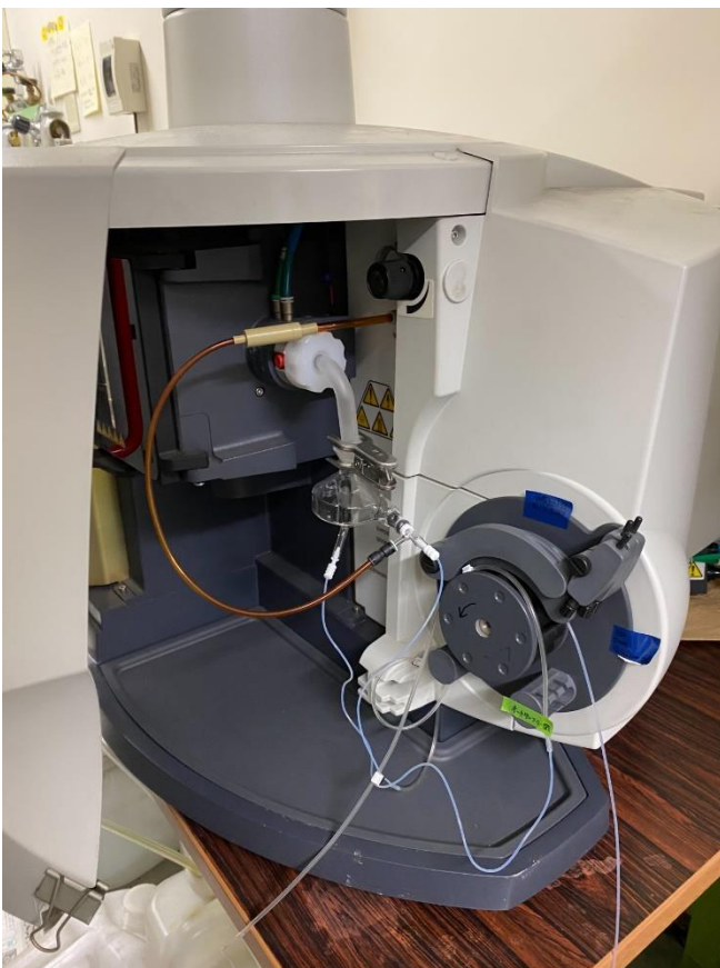
Figure 24. The ThermoScientific iCAP 6200 Inductively-coupled Plasma-Optical Emission Spectrometer (ICP-OES) at the Hokkaido University was used to measure the Sr and Ca concentrations in coral skeleton
