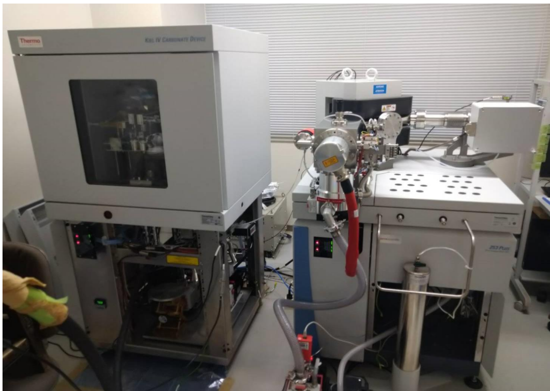
Figure 25. The Finnigan MAT 253plus stable isotope ratio mass spectrometer with the Kiel IV automated carbonate device was used to measure oxygen ( \delta^{18}\text{O} ) and carbon ( \delta^{13}\text{C} ) isotopes in coral skeleton.
