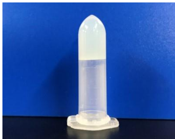
Figure S1. Digital photograph of the precursor of OEG/PAAm DN hydrogel (OEG gel with AAm monomer). The OEG and MBAA concentrations in the gel were 5 wt.% and 0.1% of AAm in moles, respectively.
