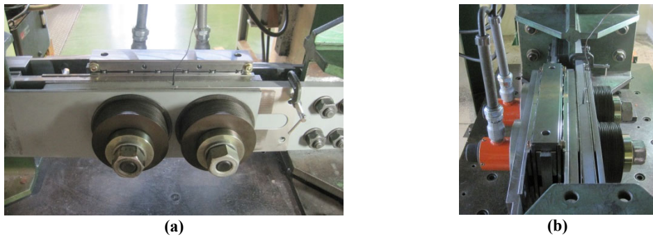
Figure 3 Photographs of the elemental test specimen consisting of two variable friction damper (VFD) units: (a) front view 43 ; and (b) side view
