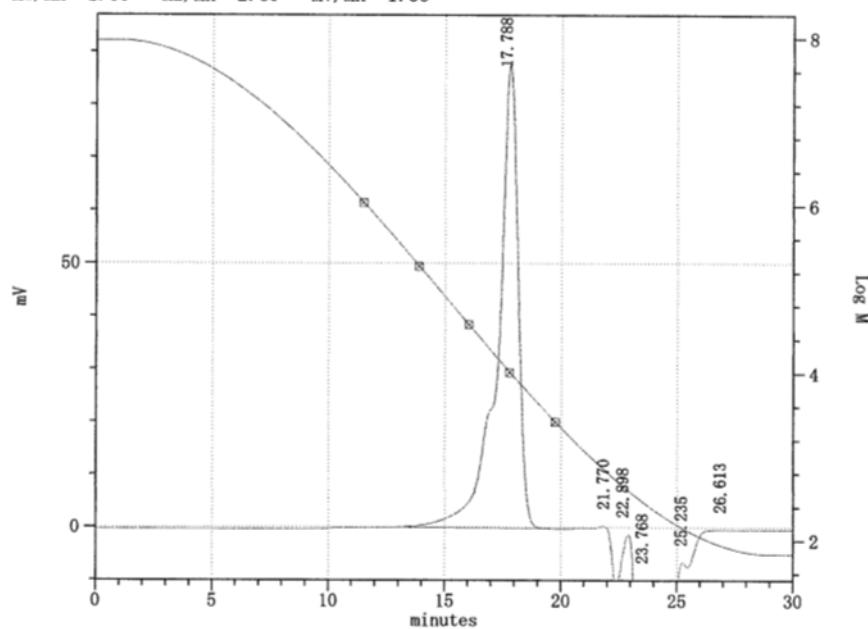
**Figure S-6.** *n*-BuLi Initiated Polymerization of Styrene in The Flow System (flow rate of *n*-BuLi (0.05 M) = 1.0 mL/min, flow rate of Styrene (2.0 M) = 2.0 mL/min, T-250-250 mixer, 30 degree-C)
