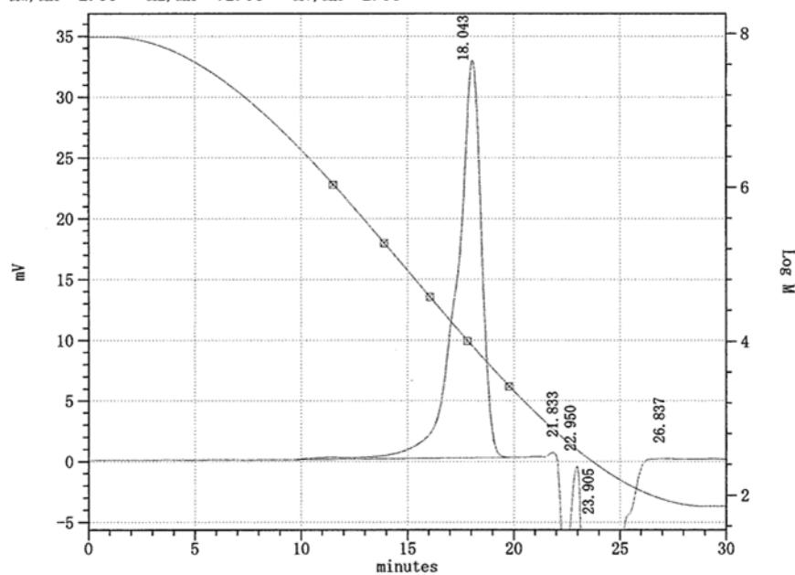
**Figure S-45.** *n*-BuLi Initiated Polymerization of Styrene in The Flow System (flow rate of *n*-BuLi (0.05 M) = 1.0 mL/min, flow rate of Styrene (2.0 M) = 2.0 mL/min, T-500-250 mixer, 30 degree-C)
