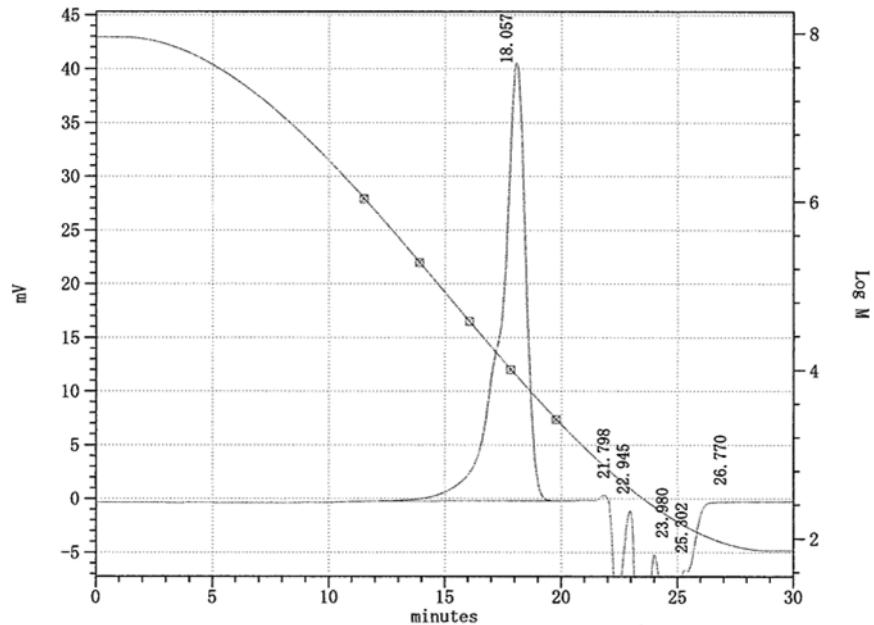
**Figure S-38.** *n*-BuLi Initiated Polymerization of Styrene in The Flow System (flow rate of *n*-BuLi (0.05 M) = 1.0 mL/min, flow rate of Styrene (2.0 M) = 2.0 mL/min, T-250-500 mixer, 30 degree-C)
