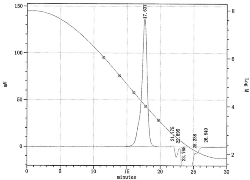
**Figure S-15.** *n*-BuLi Initiated Polymerization of Styrene in The Flow System (flow rate of *n*-BuLi (0.05 M) = 7.5 mL/min, flow rate of Styrene (2.0 M) = 15.0 mL/min, T-250-250 mixer, -20 degree-C)
