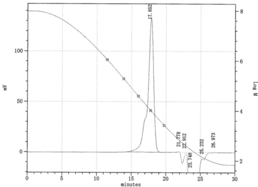
**Figure S-24.** *n*-BuLi Initiated Polymerization of Styrene in The Flow System (flow rate of *n*-BuLi (0.05 M) = 3.0 mL/min, flow rate of Styrene (2.0 M) = 6.0 mL/min, T-500-500 mixer, 30 degree-C)
