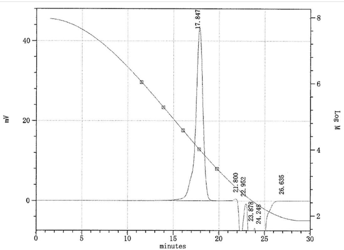
**Figure S-53.** *n*-BuLi Initiated Polymerization of Styrene in The Flow System (flow rate of *n*-BuLi (0.05 M) = 7.5 mL/min, flow rate of Styrene (2.0 M) = 15.0 mL/min, T-250-250 mixer, 30 degree-C, 2<sup>nd</sup> trial)
