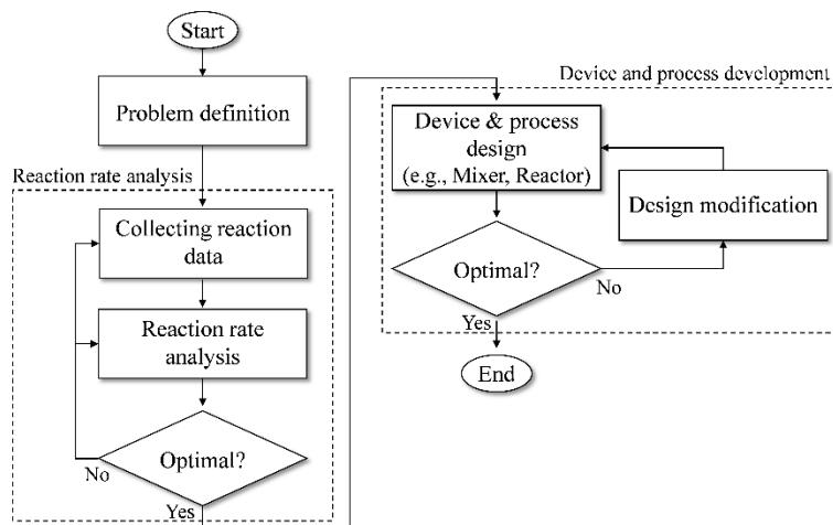
**Figure 1.** Flowchart of developing chemical processes
