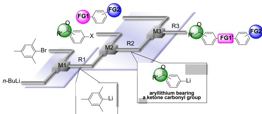
**Figure 4.** A flow microreactor system for the reaction of aryllithium bearing a ketone carbonyl group generated by iodine–lithium exchange with aromatic compounds having different electrophilic functional groups.
