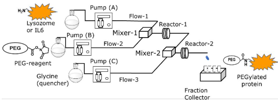
**Figure 1.** Flow diagram of continuous flow protein PEGylation.
