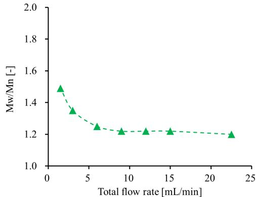
**Figure 2.** Relationship between total flow rate and Mw/Mn
