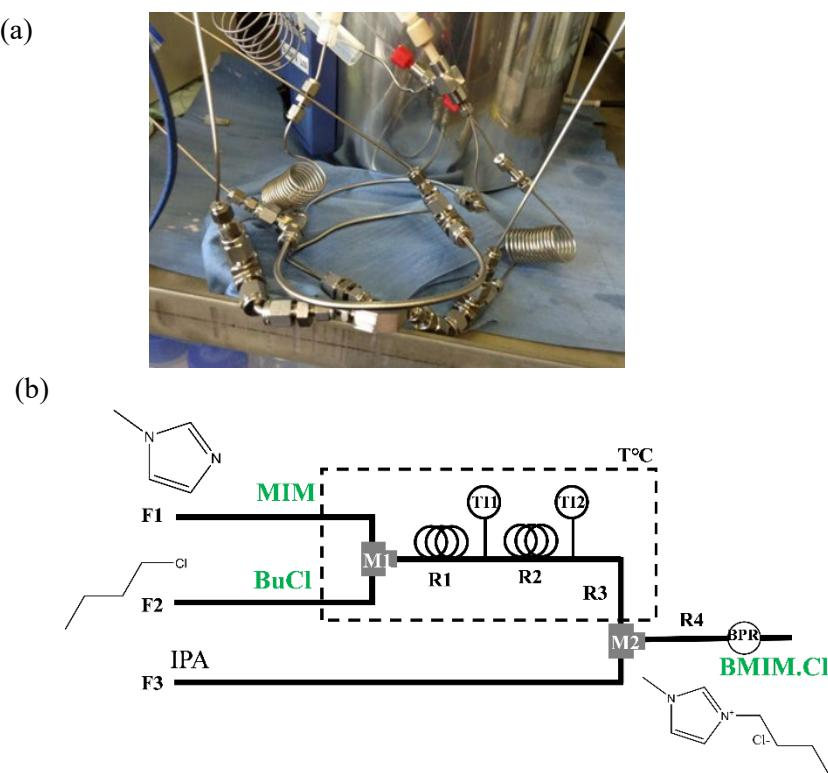
**Figure 2.** FMR-based experimental system: (a) photo of the part immersed in the oil bath and (b) process flow diagram.
