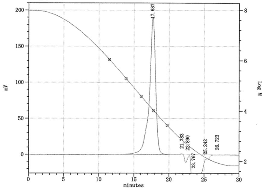
**Figure S-17.** *n*-BuLi Initiated Polymerization of Styrene in The Flow System (flow rate of *n*-BuLi (0.05 M) = 4.0 mL/min, flow rate of Styrene (2.0 M) = 8.0 mL/min, T-250-250 mixer, -20 degree-C)
