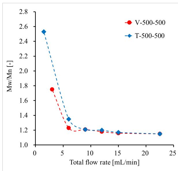
**Figure 7.** Comparing V-shape and T- shape mixers
