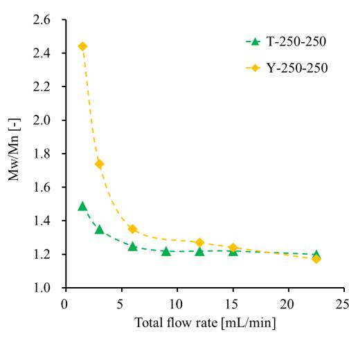
**Figure 8.** Comparing Y-shape and T- shape mixers
