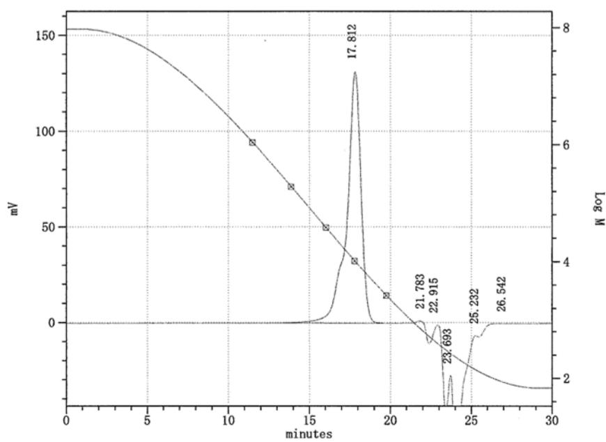
**Figure S-29.** *n*-BuLi Initiated Polymerization of Styrene in The Flow System (flow rate of *n*-BuLi (0.05 M) = 4.0 mL/min, flow rate of Styrene (2.0 M) = 8.0 mL/min, Y-250-250 mixer, 30 degree-C)
