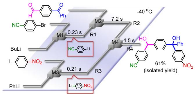
**Figure 5.** Chemosselective three-component coupling using an integrated flow microreactor system
