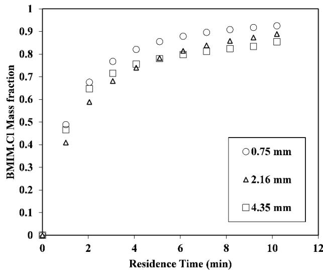
**Figure 9.** ILs synthesis profiles on tubular diameter
