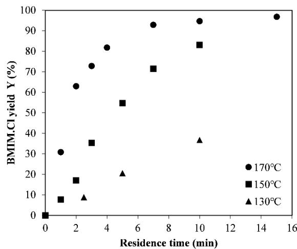
**Figure 3.** Yield profiles of ILs synthesis at different temperatures
