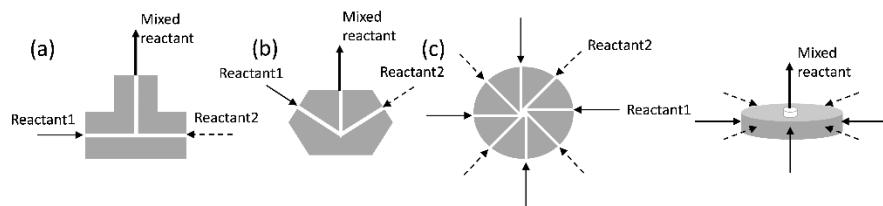
**Figure 6.** Schematic diagram of mixers: (a) T-shaped mixer (0.5 mm I.D.), (b) V-shaped mixer (0.5 mm I.D.), (c) Vortex shaped mixer (0.45 mm I.D.)
