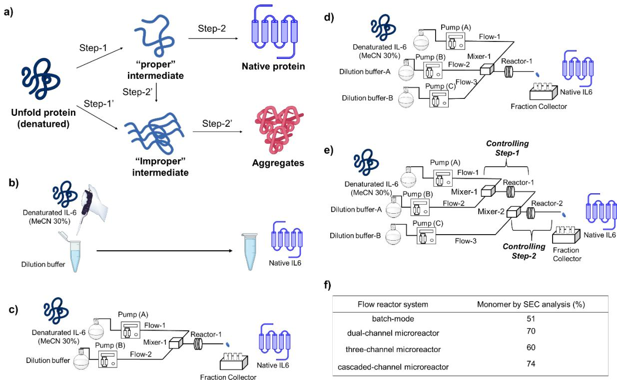
**Figure 1.** Overview of FMR mode refolding, a) illustration of “proper” and “improper” intermediates b) illustration of batch-mode refolding system, c) illustration of FMR refolding system using a dual-channel microreactor, d) illustration of FMR refolding system using a triple-channel microreactor, e) illustration of FMR refolding system using a cascaded-channel microreactor, f) Summary of feasibility study results
