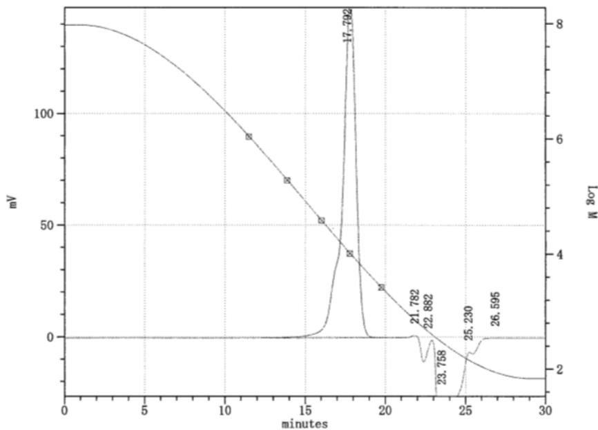
**Figure S-28.** *n*-BuLi Initiated Polymerization of Styrene in The Flow System (flow rate of *n*-BuLi (0.05 M) = 5.0 mL/min, flow rate of Styrene (2.0 M) = 10.0 mL/min, Y-250-250 mixer, 30 degree-C)
