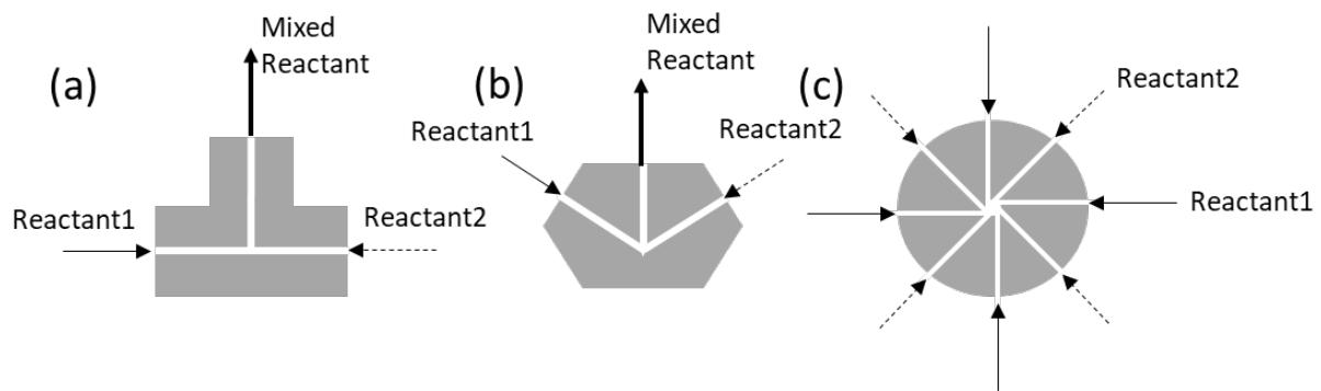
**Figure S3.** (a) T-shaped mixer ( $\phi$  500  $\mu\text{m}$ ), (b) V-shaped mixer ( $\phi$  500  $\mu\text{m}$ ), (c) vortex shaped mixer ( $\phi$  450  $\mu\text{m}$ ) in vortex shaped mixer, each reactant was divided by 4 feeding lines.
