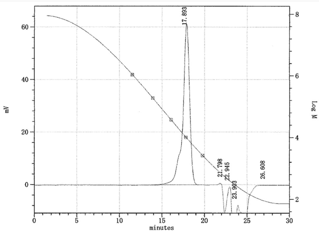
**Figure S-55.** *n*-BuLi Initiated Polymerization of Styrene in The Flow System (flow rate of *n*-BuLi (0.05 M) = 4.0 mL/min, flow rate of Styrene (2.0 M) = 8.0 mL/min, T-250-250 mixer, 30 degree-C, 2<sup>nd</sup> trial)
