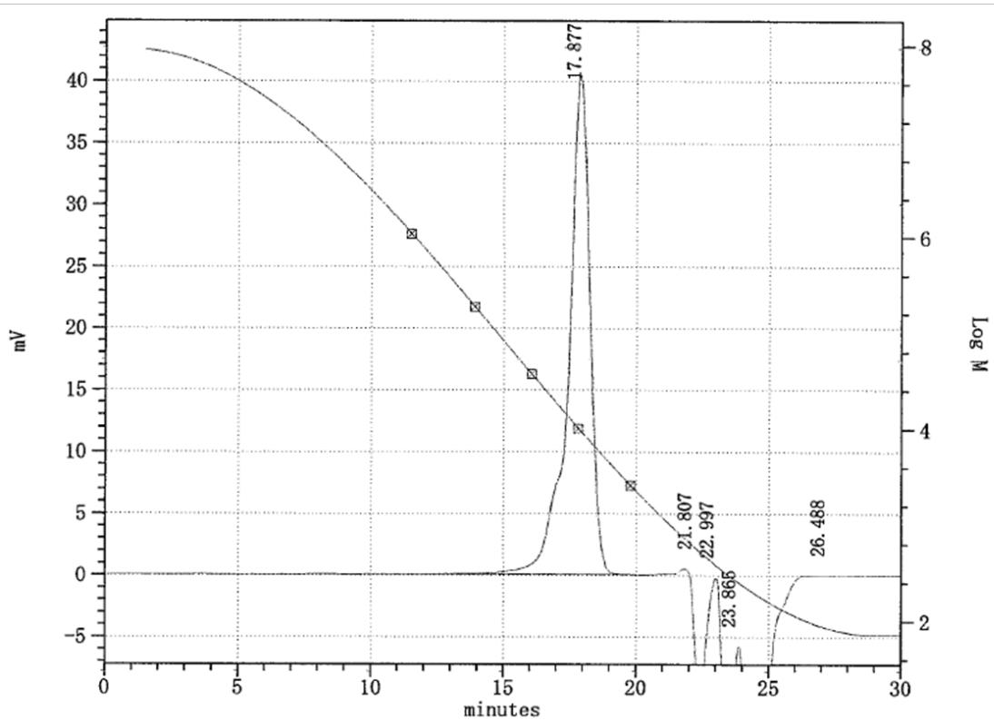
**Figure S-54.** *n*-BuLi Initiated Polymerization of Styrene in The Flow System (flow rate of *n*-BuLi (0.05 M) = 5.0 mL/min, flow rate of Styrene (2.0 M) = 10.0 mL/min, T-250-250 mixer, 30 degree-C, 2<sup>nd</sup> trial)
