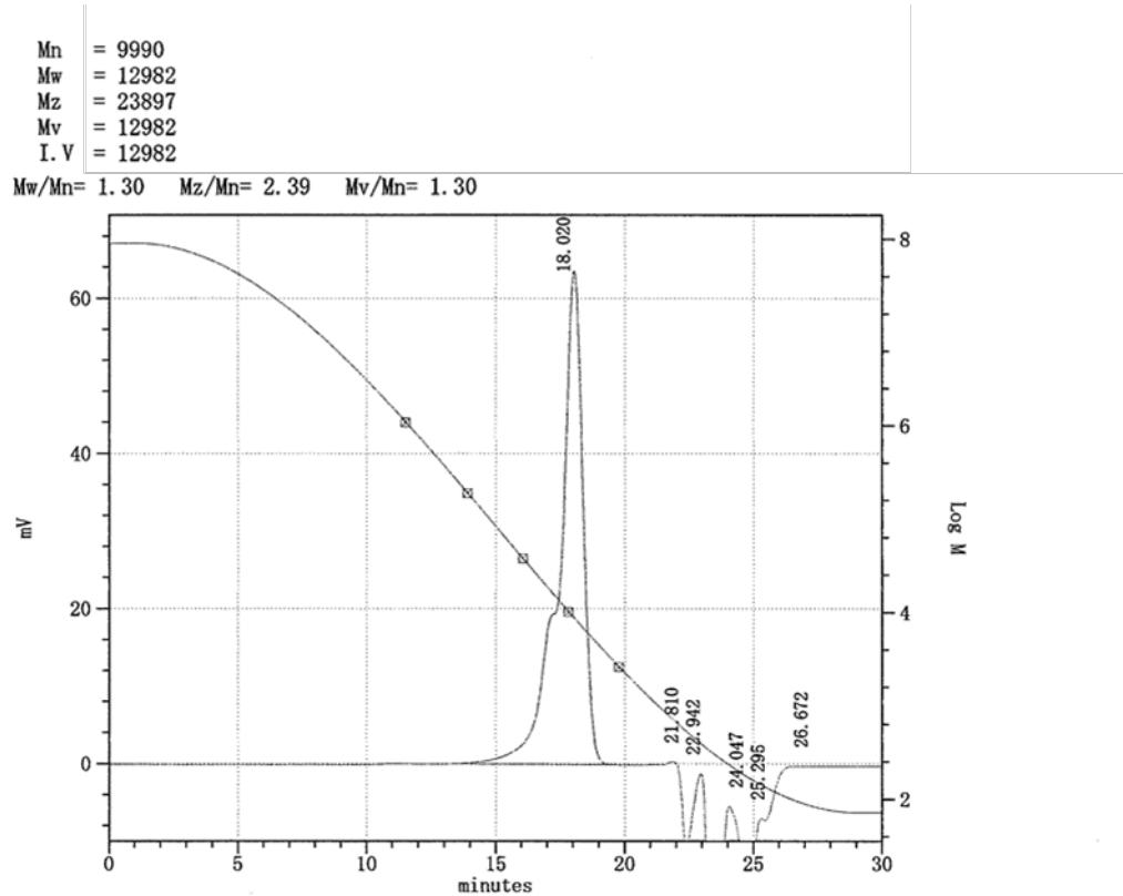
**Figure S-37.** *n*-BuLi Initiated Polymerization of Styrene in The Flow System (flow rate of *n*-BuLi (0.05 M) = 2.0 mL/min, flow rate of Styrene (2.0 M) = 4.0 mL/min, T-250-500 mixer, 30 degree-C)
