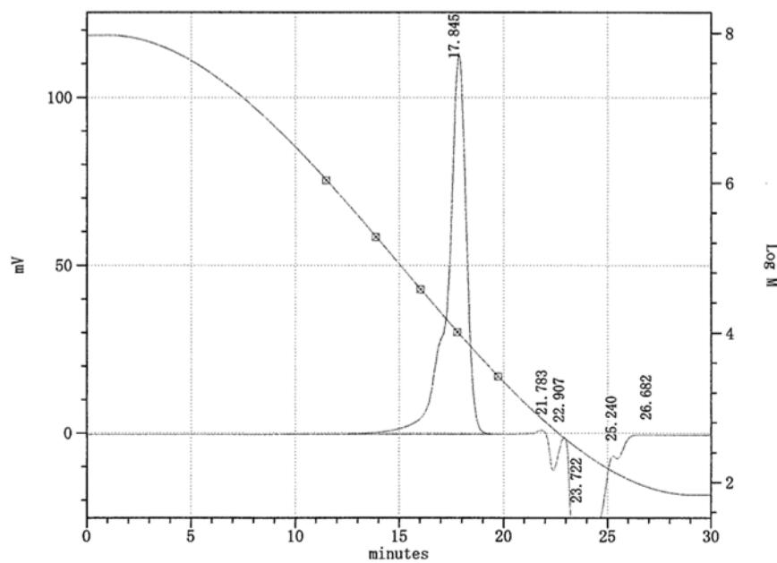
**Figure S-30.** *n*-BuLi Initiated Polymerization of Styrene in The Flow System (flow rate of *n*-BuLi (0.05 M) = 2.0 mL/min, flow rate of Styrene (2.0 M) = 4.0 mL/min, Y-250-250 mixer, 30 degree-C)
