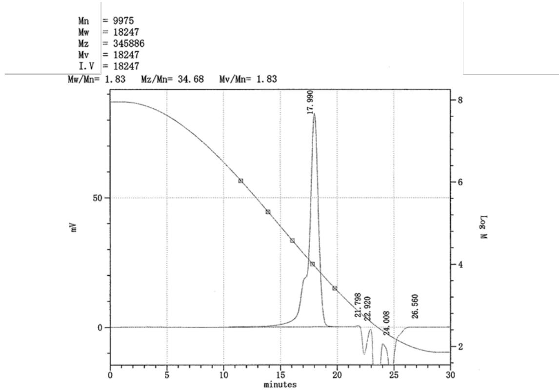
**Figure S-43.** *n*-BuLi Initiated Polymerization of Styrene in The Flow System (flow rate of *n*-BuLi (0.05 M) = 3.0 mL/min, flow rate of Styrene (2.0 M) = 6.0 mL/min, T-500-250 mixer, 30 degree-C)
