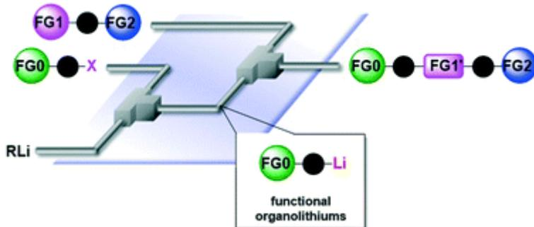
**Figure 1.** Illustration of chemoselective reactions of difunctional electrophiles with functional aryllithiums induced by micromixing
