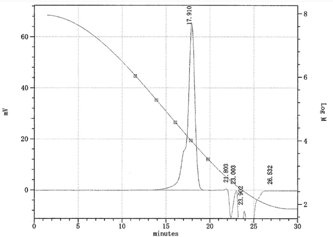
**Figure S-57.** *n*-BuLi Initiated Polymerization of Styrene in The Flow System (flow rate of *n*-BuLi (0.05 M) = 2.0 mL/min, flow rate of Styrene (2.0 M) = 4.0 mL/min, T-250-250 mixer, 30 degree-C, 2<sup>nd</sup> trial)
