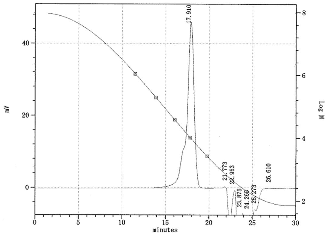
**Figure S-56.** *n*-BuLi Initiated Polymerization of Styrene in The Flow System (flow rate of *n*-BuLi (0.05 M) = 3.0 mL/min, flow rate of Styrene (2.0 M) = 6.0 mL/min, T-250-250 mixer, 30 degree-C, 2<sup>nd</sup> trial)
