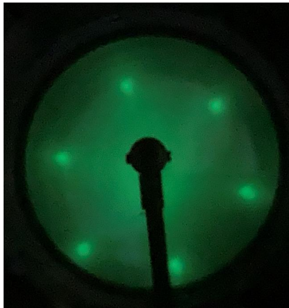
Figure 3-1. (1 \times 1) LEED pattern of Co(0001) clean surface, probe electron energy = 150 eV.
