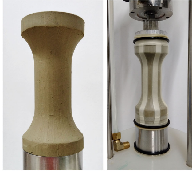
(b) Specimen, as trimmed, and as enclosed by rubber membrane with filter paper strips
