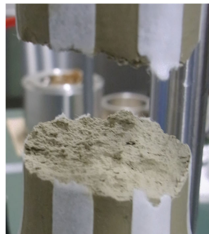
(b) Test 22: Typical rupture surface
