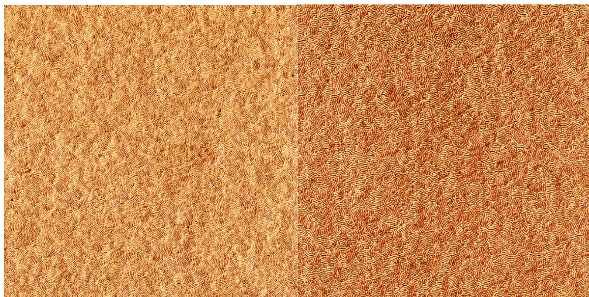
Figure S5.22. AFM phase images of (a) S_{65}BS_{28}(cl)-LA_{160} and (b) S_{65}BS_{28}(cl)-LA_{223} thin films on the PS_{0.2}\text{-stat-}PMMA_{0.8} brush underlayer. The images are 5\ \mu\text{m} square.
