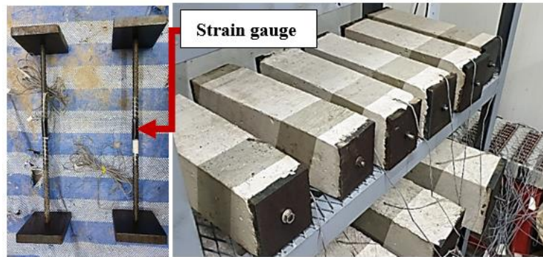
Figure 3.1 Specimens for length change measurement in restrained condition
