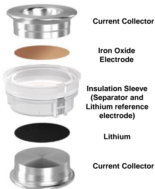
Figure 6.2 Schematic of lithium ion battery half-cell.
