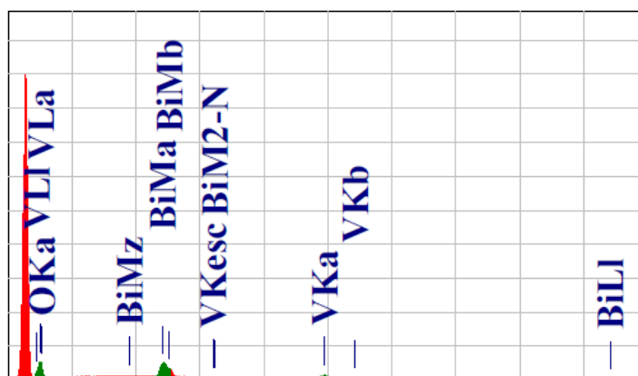
Figure 2.6. EDS of BVO NFs A. The highest peak on the left is the carbon peak originating from the carbon tape which was used as the substrate for attaching samples. The calculated Bi/V/O ratio is 1/1.2/3.7, which is pretty close to the stoichiometric ratio of \text{BiVO}_4 . No Na atom's related signal can be observed from the EDS measurement.
