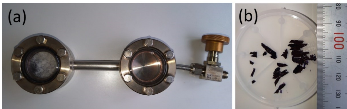
Figure 2-11. (a) Scaling up of the growth apparatus. (b) Obtained pentacene crystals.
