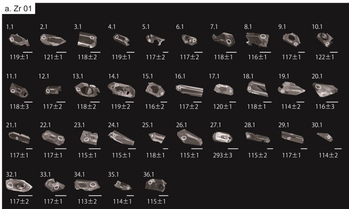
Fig. 5 Cathodoluminescence images of zircon grains from studied samples. See Zr in Fig. 1-d for their horizons. a: Zr 01 and b: Zr 02 recording analysis spots and U-Pb ages (in Ma); ages are based on ^{206}\text{Pb}/^{238}\text{U} ages. Scale bars are 50 \mu\text{m} .
