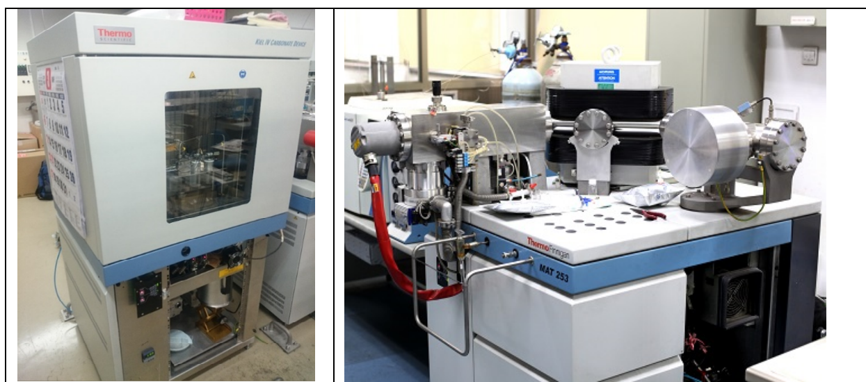
Figure 2.4. The Finnigan MAT 253 mass spectrometer with an automatic carbonate device (Kiel IV) in Hokkaido University.
