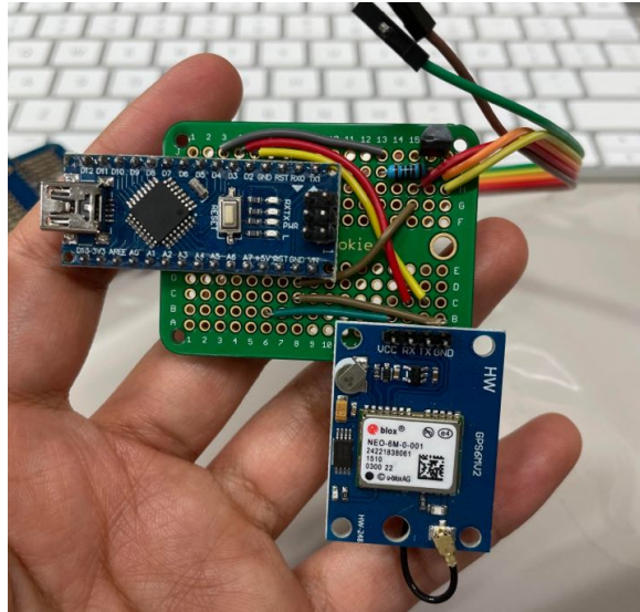
Figure 2.5 Implemented circuit for ground camera synchronized capture time.
