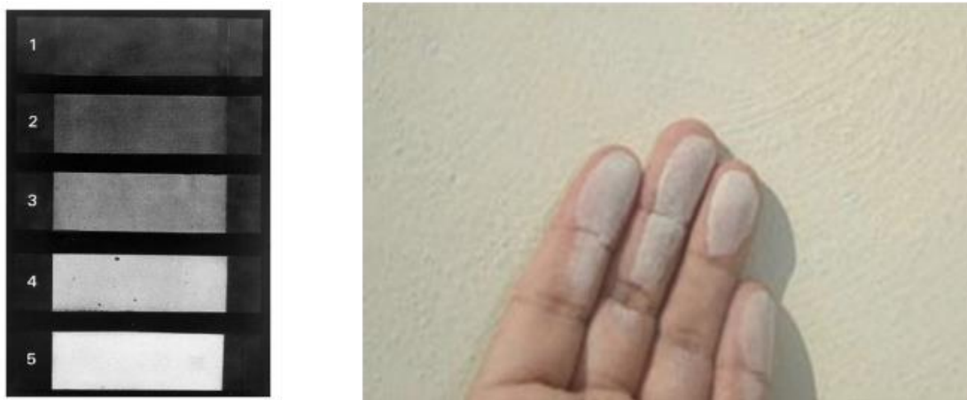
Figure 3.22 Chalking pictorial standards (ISO 4628-6&7)
