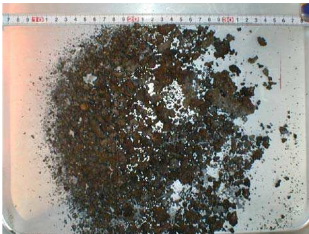
Figure 4.8 Photograph of appearance of desulfurization slag after treatment (condition A)
